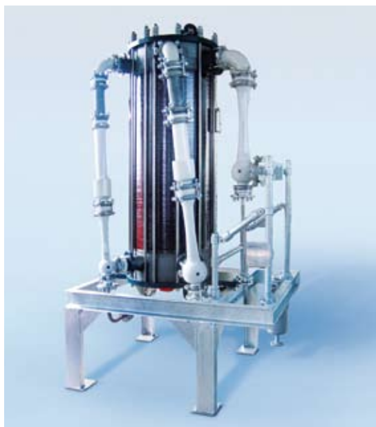
Fig. 3 4-stage steam jet vacuum pump with surface condenser Materials: porcelain and graphite Suction capacity: 22.7 kg/h from 16 mbar abs.
