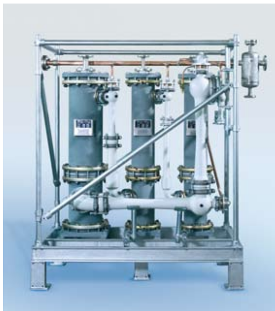
Fig. 2 5-stage steam jet vacuum pump in corrosion-resistant design Materials: jet pump in porcelain, mixing condensers in C-steel enamelled Suction capacity: 5 kg/h of air from 2.5 mbar abs.
