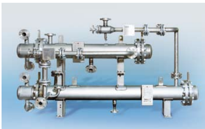
Fig. 3 2-stage steam jet vacuum pump with surface condenser, completely in Hastelloy Suction capacity: 110 kg/h from 35 mbar
